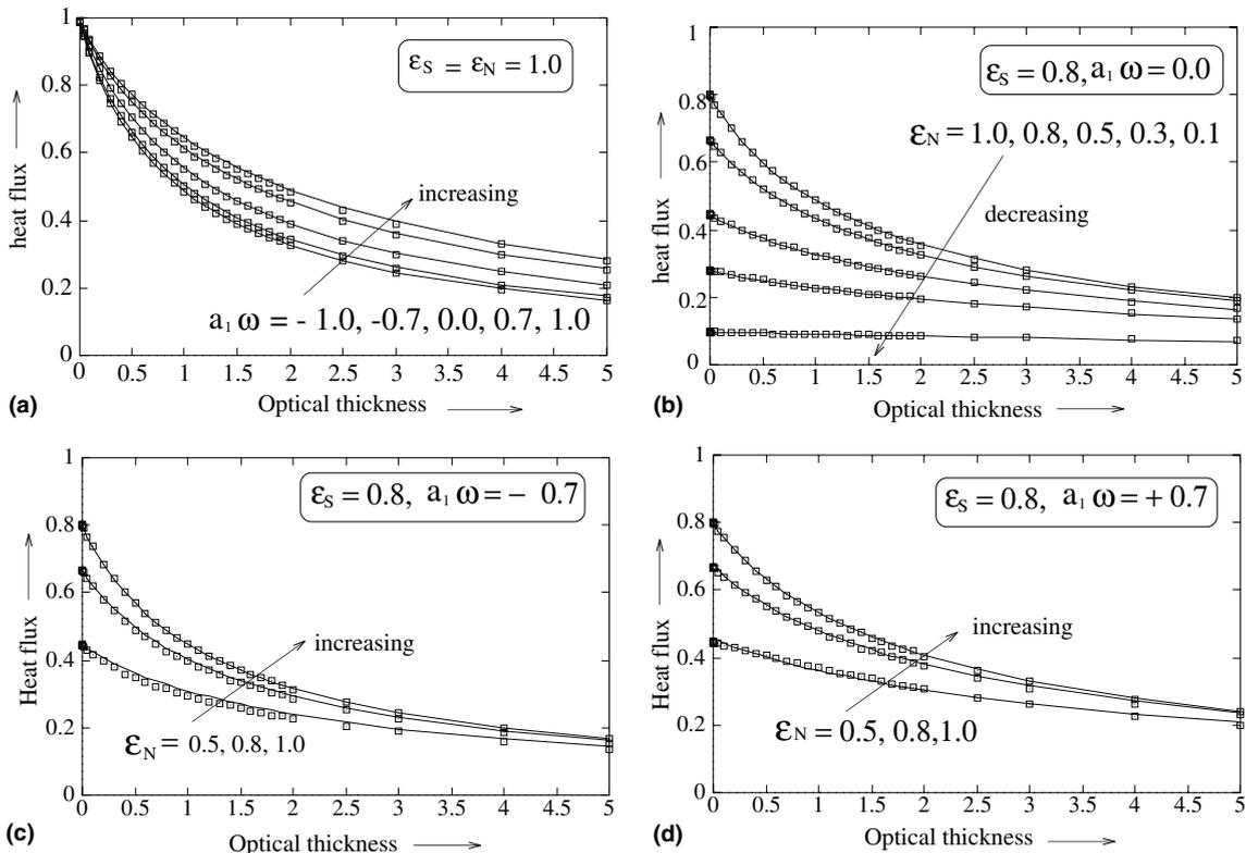
Fig. 1. Variation of non-dimensional net heat flux  $\Psi$  with enclosure optical thickness; line – CDM results, markers – Monte Carlo method results [4].
