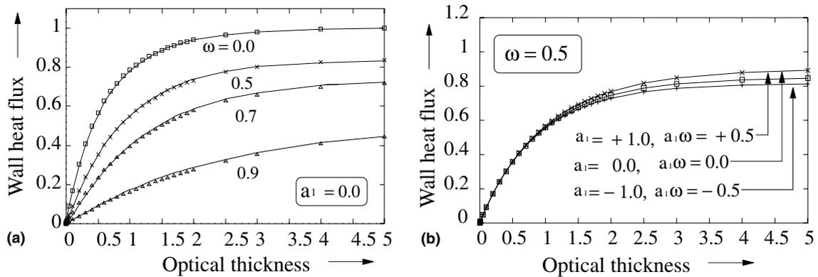
Fig. 2. Variation of non-dimensional wall heat flux  $\Psi$  with enclosure optical thickness; line – CDM results, markers – Monte Carlo method results [4].
